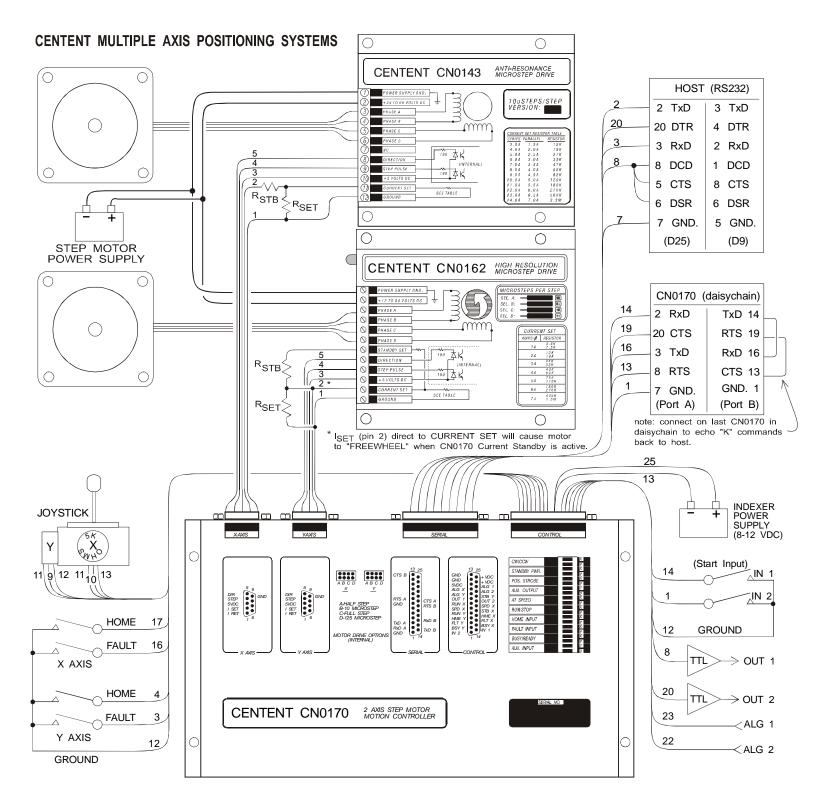
Centent step motor drivers are designed to operate 4, 6, and 8 wire motors in a low performance or a high performance configuration (a 4 wire motor is considered as high performance configuration). Please consult the driver's operating manual to determine the best configuration for your application.
