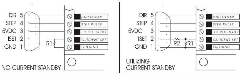
the current set resistor and R2 is the STANDBY resistor. R2 may be replaced with a wire jumper if motor current is off during standby. This allows the motor to "freewheel" with no holding torque evident. R2 is not used and ISET or IRET are not connected if current standby is not required.
