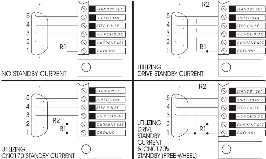
Figure 8 shows the possible configurations for connecting the CN0162 to the CN0170. R1 is the current set resistor and R2 is the STANDBY resistor. Refer to the Operating Manual, CN0162 Microstep Drive to determine the values for R1 and R2.
