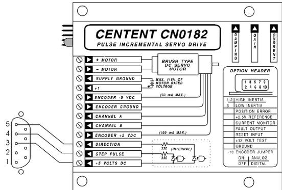
Figure 10, CN0182 connections
