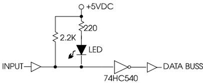
Figure 14, Input circuit
