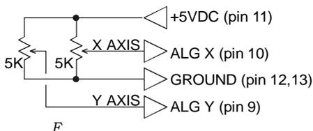
Figure 16, Joystick interface
