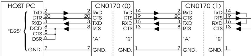
Figure 18, D25 RS232 connections
